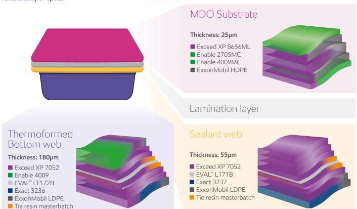
Exceed Sperformance polyethylene can also be used in both the thermoformed web as well as the MDO film/sealant film and provide excellent stiffness/toughness/formability. Please contact your ExxonMobil representative to design a tailored formulation that works best for you.
